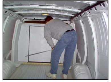
Enter rear floor panel VLS 004 through side door opening and position so the tongue of the floor is under the rear door frame. Note: Make sure the steel at the bottom of the door frame is tucked under the grey polyboard on rear floor panel. Install 3/16" rivets supplied.
