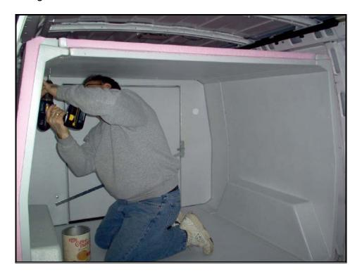
Secure VLS009 and VLS010 to roof panel with # 10 x 2.5 pan head screw.
