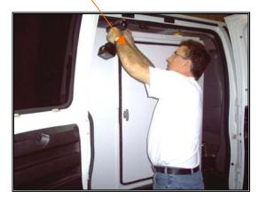
Use sealant (supplied) to seal all joints in the body. Allow sealant to cure properly as per manufacturer's instruction on sealant cartridge.
