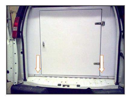
Secure 11.5" side wall panels to floor with 2 screws #12 x 2.5 inches waferhead plated. Make sure the outside installer is pushing the back of the 11.5" side panels inwards as the inside installer is drilling the holes to ensure tightest possible joint.
