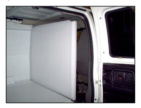
Enter side door panel part # VLS011 and locate with curbside wheel arch panel and floor. Secure with #10 x 2.5" panhead screws on inside of door panel only.
