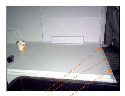
To secure the kit to the van - Drill 3 holes, 5/32", in the front flange of the front floor panel (these holes should be in line with the ribs in the floor of the van and make sure you are not drilling into anything underneath the van) and secure with 3 #12 wafer head screws.
