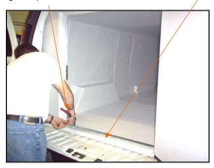
Rivet finishing angle at top of door frame as shown below.
