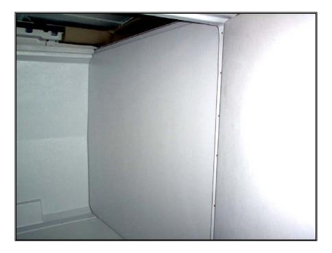
When bulkhead is in position the second installer in the drivers cab, holes should only be drilled and screwed down both sides of the bulkhead for the moment. (see below)
