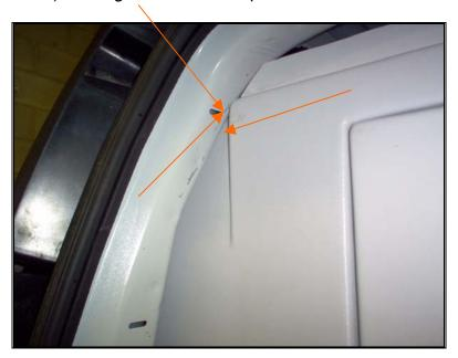
Insert front bulkhead part # VLS 005 through side door opening and rest against back of seats.
