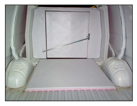
Outside installer should secure with 2 panhead screws x 2.5", locating holes (shown below) have to be drilled through with 5/32 inch drill.
