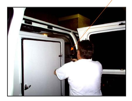
Secure side door panel assembly to floor and roof with #10 x 2.5" pan head screws.
