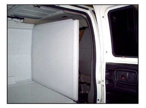
Enter side door panel part # VLS011 and locate with curbside wheel arch panel and floor. Secure with #10 x 2.5" panhead screws on inside of door panel only.
