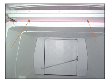
1. Secure 20" floor extension panel VLS 019 to VLS 004 floor panel with waferhead screws.
