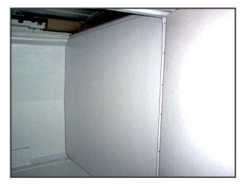
When bulkhead is in position the second installer in the drivers cab, holes should only be drilled and screwed down both sides of the bulkhead for the moment. (see below)
