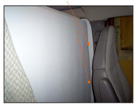
Slide front roof panel (which was stored above rear roof panel) forward and locate with front drivers side wall panel (fuel filler panel) and side door frame. Secure with  $#10 \times 2.5$ " panhead screws.
