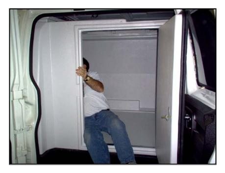
With second installer in the drivers cab, locate bulkhead into position now with floor panel, fuel filler panel, and side door frame.
