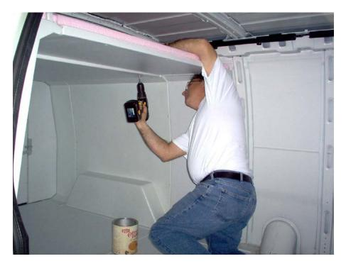
Enter front drivers side wall (fuel filler panel) part # VLS006 through side door opening and locate, secure with 2 # 10 2.5" panhead screws at <u>rear only.</u> Holes are to be drilled with 5/32 inch drill.
